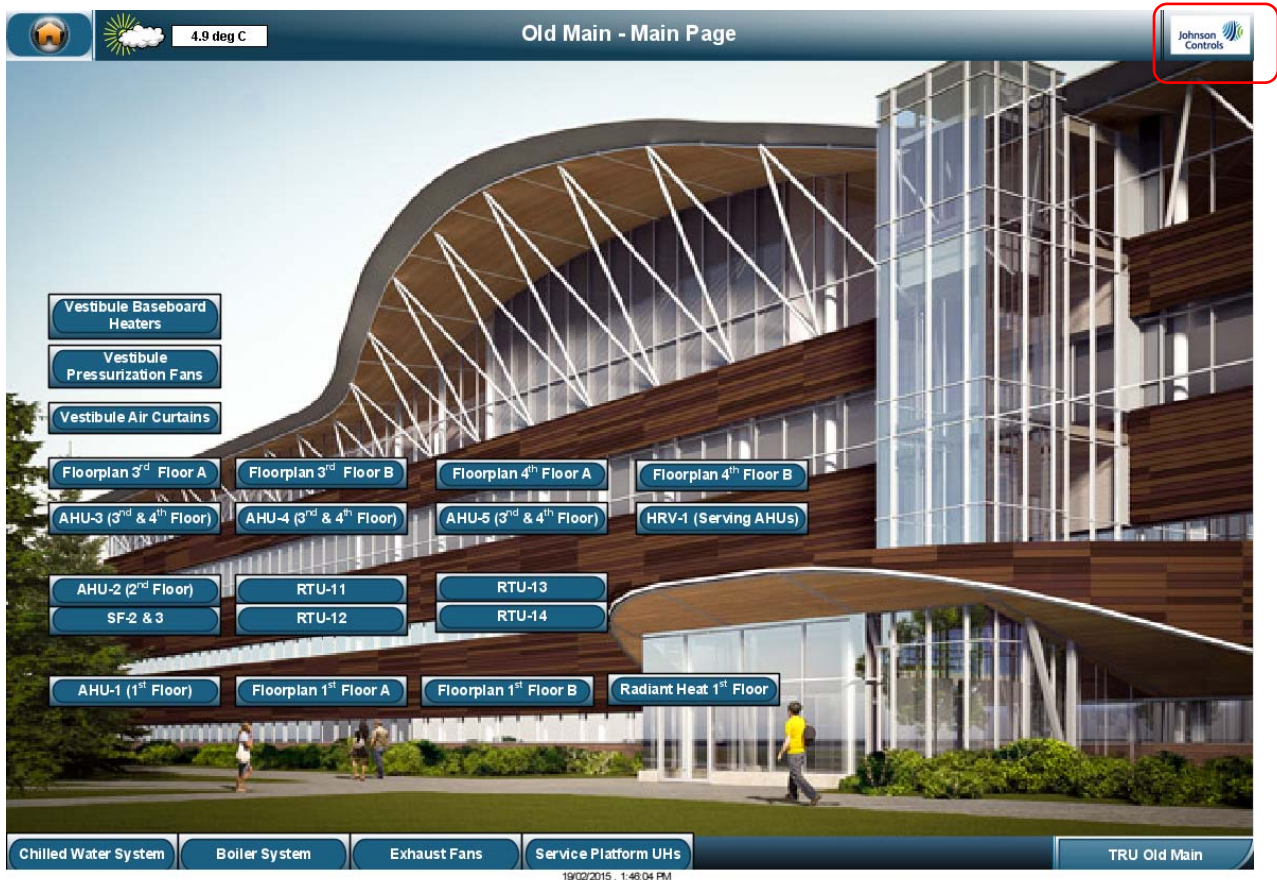
Figure 14: Johnson Controls BAS Graphic
